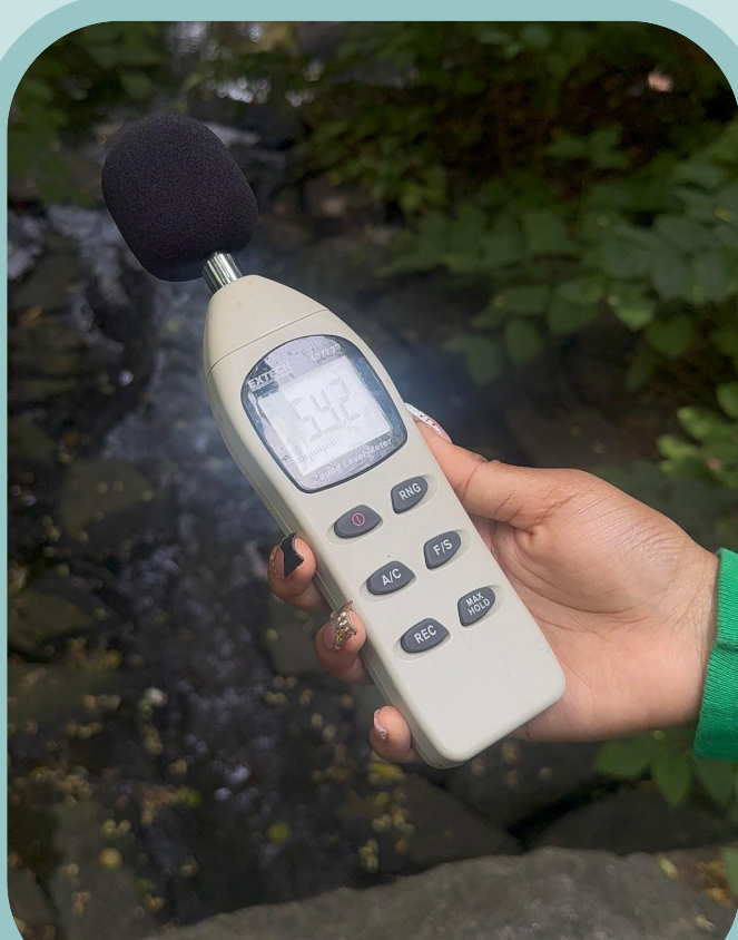
Image 2. Close Up of Extech Digital Sound Level Meter used for interval ambient noise surveys
